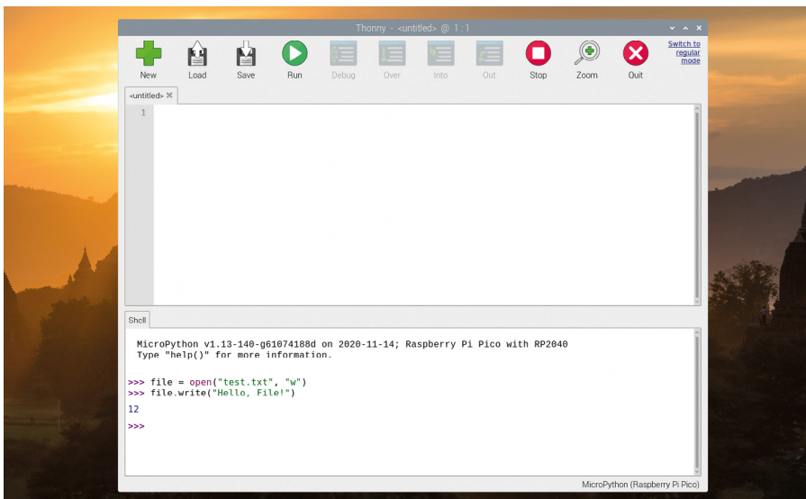
▲ Figure 9-1: The size of the data you've written is printed to the Shell area
